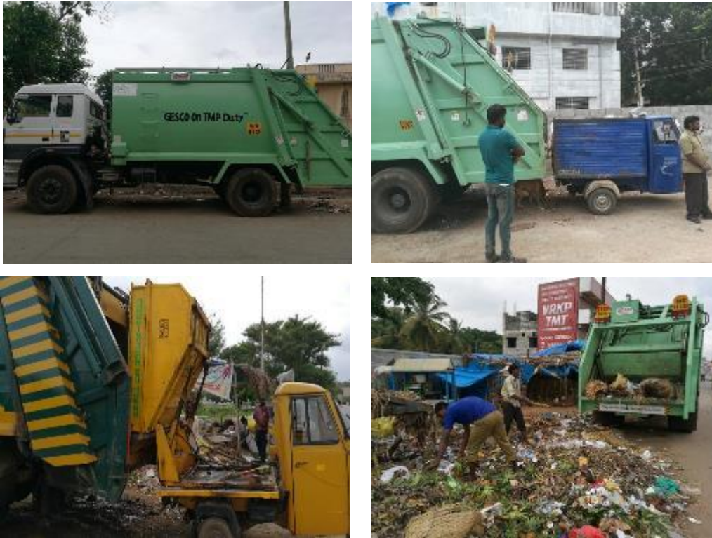
Figure 5: Secondary Collection & Transportation by Compactors
